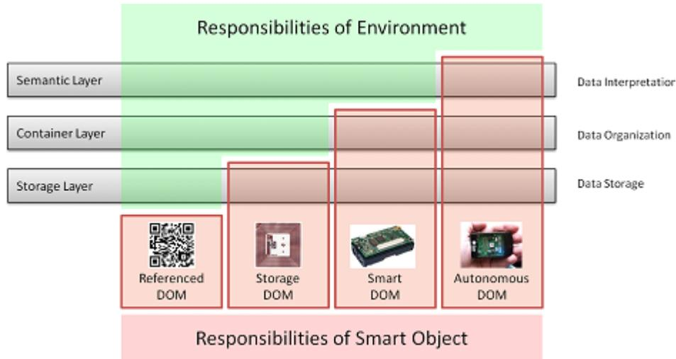
**Figure 2:** Layered Memory Architecture and Resulting Sharing of Responsibilities between Smart Object and Environment for Basic Memory Classes.
