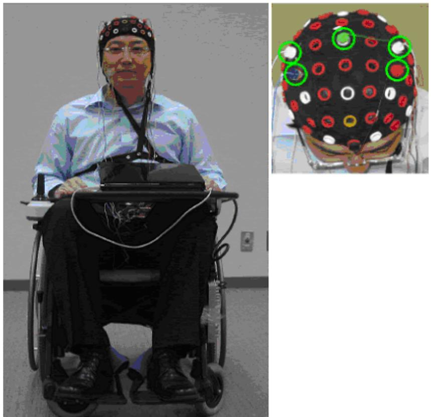
**Figure 7:** Motorized Wheelchair driven by BCI Technology, from Toyota.
