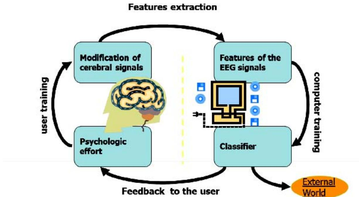
Figure 2: Logical Scheme of a BCI System.
