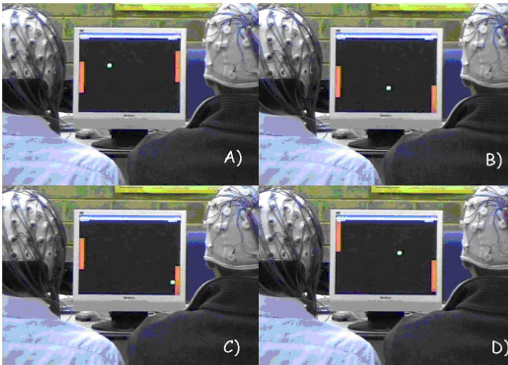
**Figure 4:** Two subjects playing electronic ping-pong without moving muscles, by means of a brain-computer interface installed at *Fondazione Santa Lucia* in Rome, Italy. (Panels run from A) to D).)
